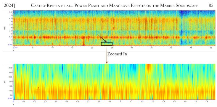
FIG. 2. Spectrogram of Point A. Black arrow shows the Aguirre Power Plant Complex acoustic footprint with frequencies in the 0.01–200 Hz range with a loud rumbling sound. See Fig. 3 for zoomed acoustic footprint. Lower part is a zoomed spectrogram of the Aguirre Power Plant Complex acoustic footprint. Generated in BioRender. com.
