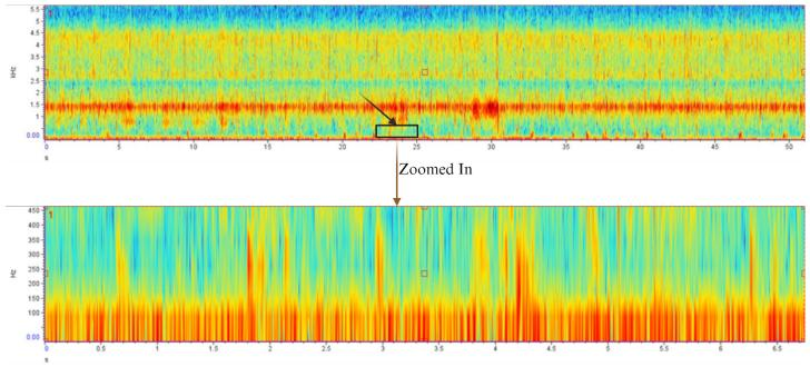
FIG. 3. Spectrogram of Point B. The black arrow shows the noise produced by the power plant is detected in the 0.01–150 Hz frequency range. Lower part is a zoomed spectrogram of the Aguirre Power Plant Complex in the 0.01–150 Hz range. Generated in BioRender.com.
