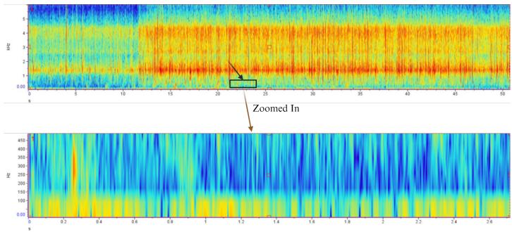
FIG. 6. Spectrogram of Point F. Black arrow shows spectral range for the Aguirre Power Plant Complex. The noise was greatly reduced in the 0.01–200 Hz frequency range. Lower part is a zoomed spectrogram that reveals the absence of the Aguirre Power Plant Complex acoustic footprint above the 100 Hz frequency range. Generated in BioRender.com.
