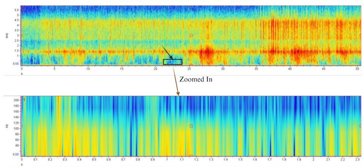
FIG. 5. Spectrogram of Point E: The black arrow points out that frequencies from the Aguirre Power Plant Complex was greatly reduced from 0.1–200 Hz to 0.01–100 Hz range at the entrance to the mangrove system. Lower part is a zoomed spectrogram of the 0.01–200 Hz frequency range in Point E which reveals reduced noise (dB of the acoustic footprint). Generated in BioRender.com.
