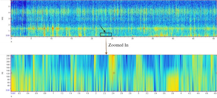
FIG. 8. Spectrogram of point H. Black arrow shows the Aguirre Power Pant Complex acoustic footprint could not be detected within the 0.01–200 Hz frequency range. Lower part is a zoomed spectrogram of the 0.01–200 Hz frequency range reveals the absence of the Aguirre Power Plant Complex acoustic footprint in Point H. Generated in BioRender.com.
