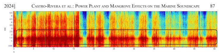
FIG. 4. Spectrogram of Point C. The black rectangle points out the noise produced by a hot water discharge tube connected to the power plant. Aguirre Power Plant Complex noise could not be detected because of spectral overshadowing. Generated in BioRender.com.
